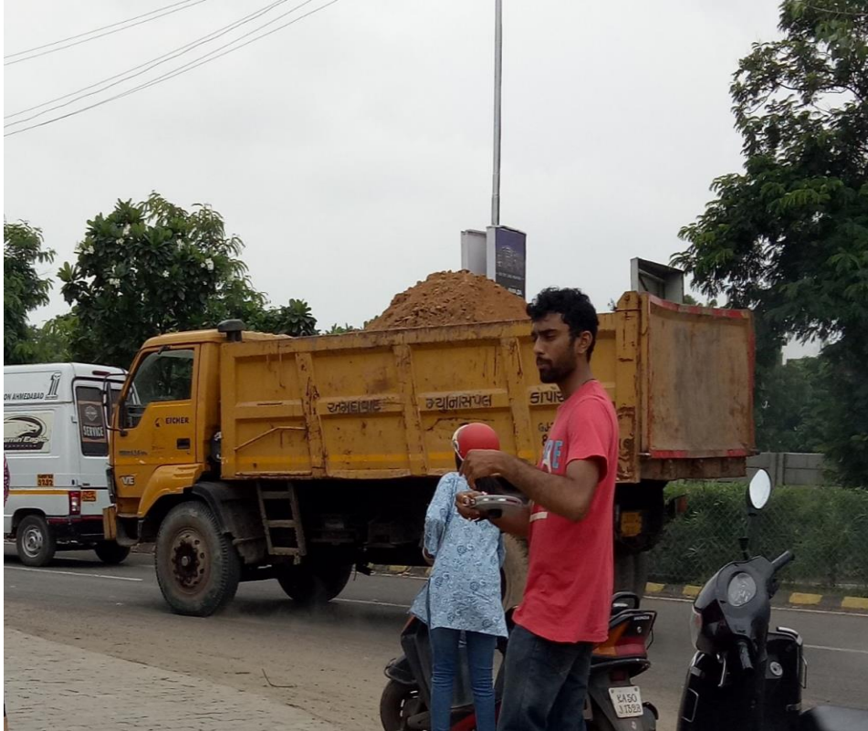
Uncovered transportation of excavated sand and materials
